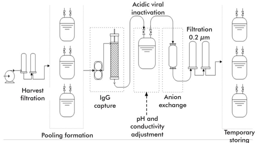
Figure 1. Downstream purification first stages flow diagram.
