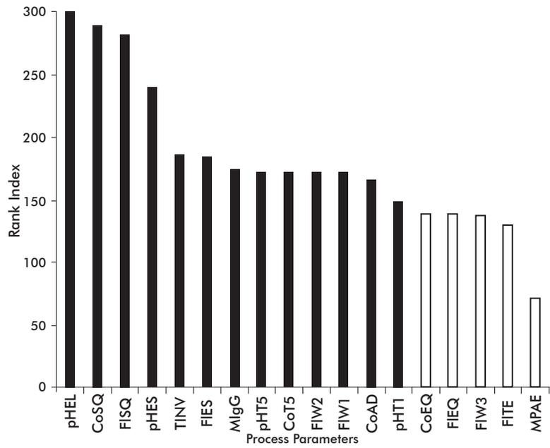
Figure 2. Pareto chart for first purification parameters criticality assessment. Bars in black stand for the most critical process parameters deduced from 80 % Pareto distribution according to cumulative percentage (81.2 %).
